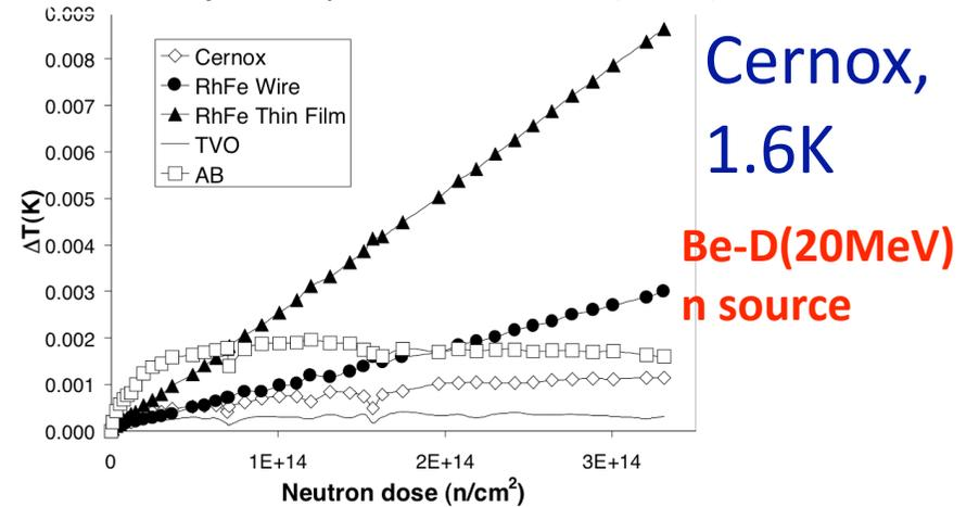
Figure 3 Error on temperature measurement on some sensors during irradiation ( $T_{bath}=1.8$  K)
