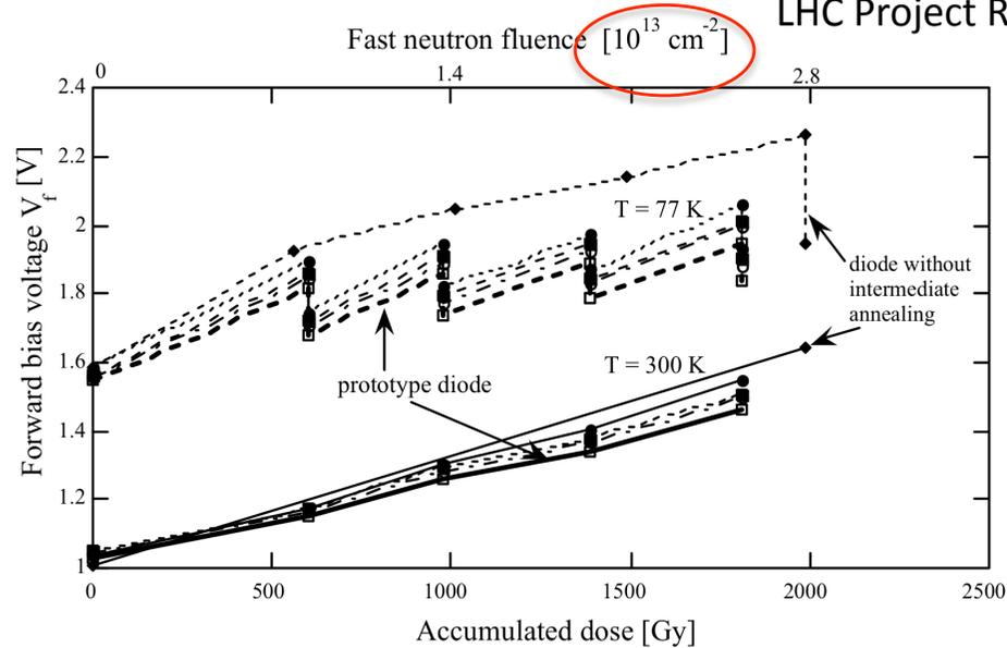
FIGURE 3. Forward bias voltage  $V_f$  at forward current  $I_f = 12 \text{ kA}$  versus accumulated dose at 77 K and 300 K for one prototype- and 3 series diodes with intermediate warm up. For comparison is also shown one diode without intermediate annealing.
