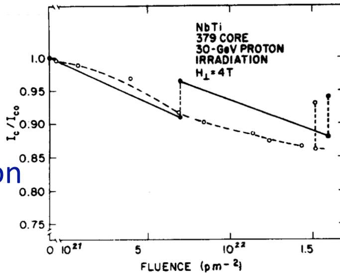
Fig. 10. Changes of critical currents measured at 4 T with proton fluence (Nb-45 wt% Ti, 379 core conductor). ○○ irradiation at 4.2 K, final anneal at room temperature; ⋯ irradiation at 4.2 K, one intermediate and one final anneal to room temperature [33].
