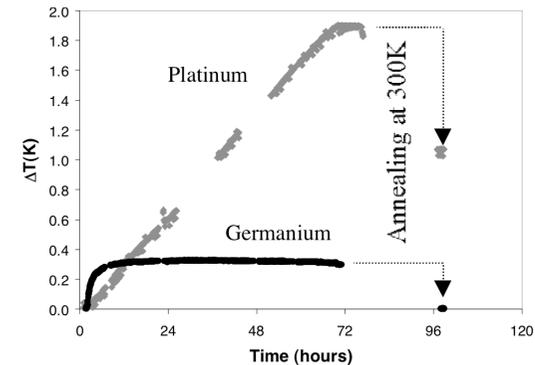
Figure 4 Irradiation-induced error on temperature read-out for Pt and Ge ( $T=1.8$  K, dose= $6 \cdot 10^{19}$  n.cm<sup>-2</sup>)
