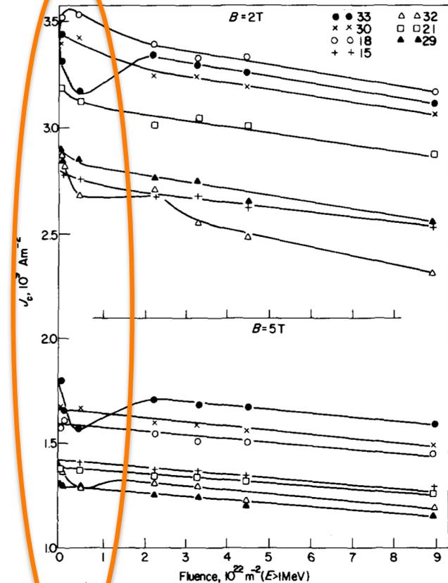
Fig. 9 Critical current densities as a function of fast neutron fluence for the seven highest  $j_c$  conductors of the present investigation
