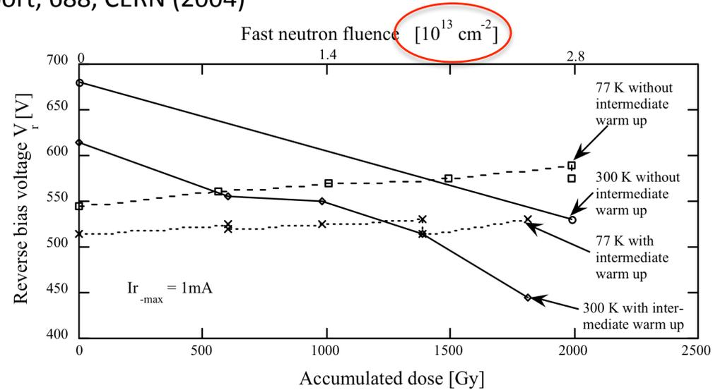
FIGURE 5. Typical reverse bias voltage  $V_r$  ( $I_r = 1 \text{ mA}$ ) at 77 K and 300 K versus accumulated dose of one diode with intermediate warm up to 300 K and one diode without intermediate warm up to 300 K.
