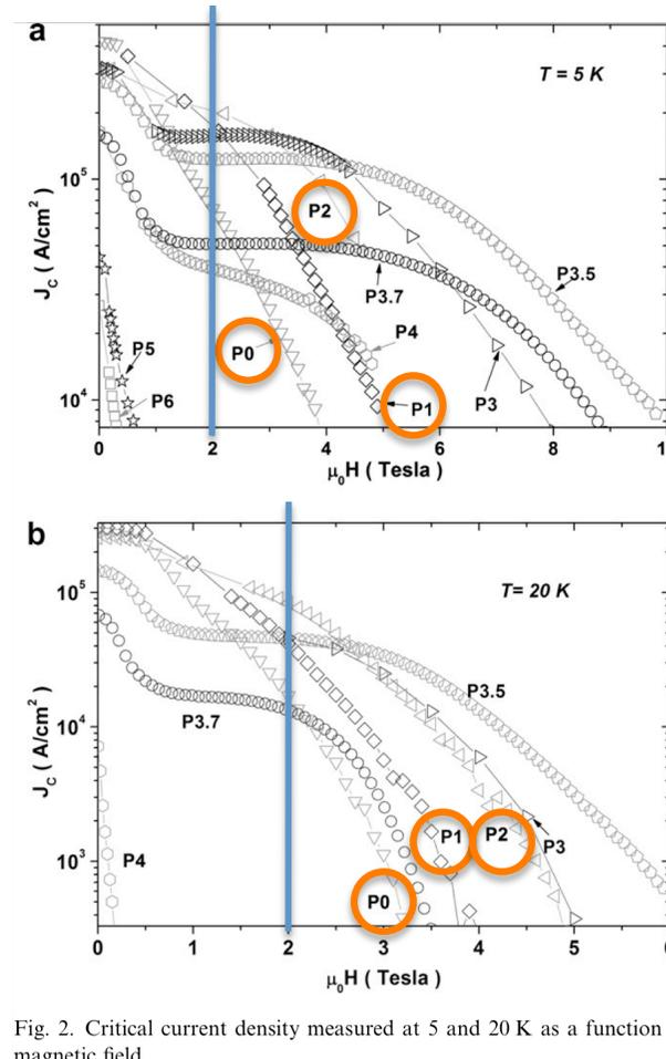
Fig. 2. Critical current density measured at 5 and 20 K as a function of magnetic field.
