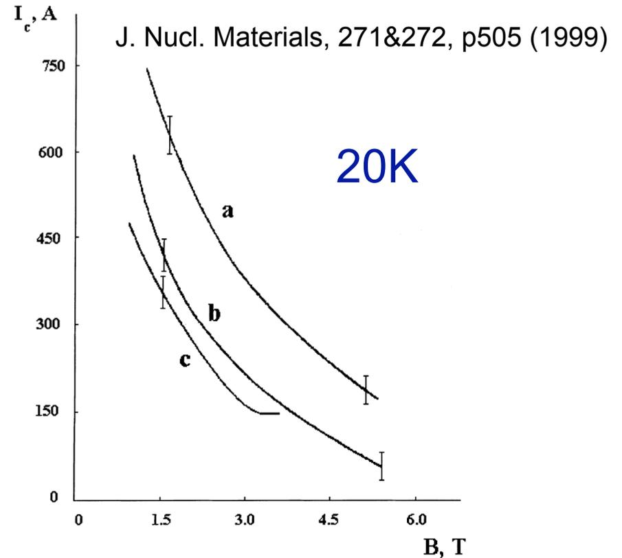
Fig. 2. Dependence of critical current vs magnetic field for 37-core industrial superconducting NbTi wire: (a) before irradiation; (b) after irradiation by the neutron fluence of  $8.6 \times 10^{17} \text{cm}^{-2}$ ; (c) after irradiation by the neutron fluence of  $1.6 \times 10^{18} \text{cm}^{-2}$ .
