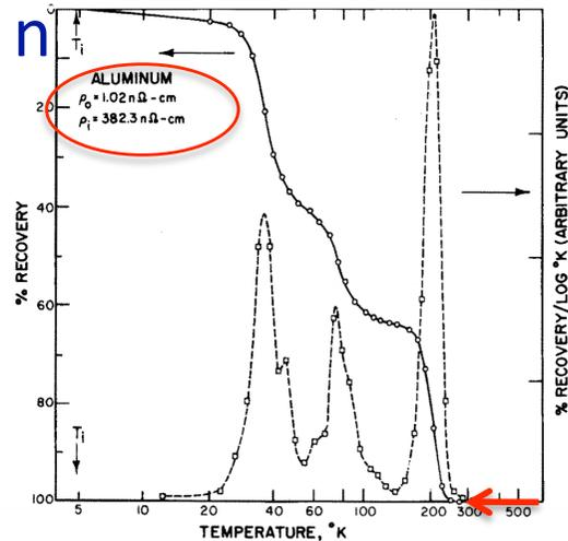
Fig. 3. Recovery and differential recovery versus logarithm of absolute temperature for aluminum irradiated at 4.5 K to  $2 \times 10^{18}$  n/cm<sup>2</sup> of  $E > 0.1$  MeV.
