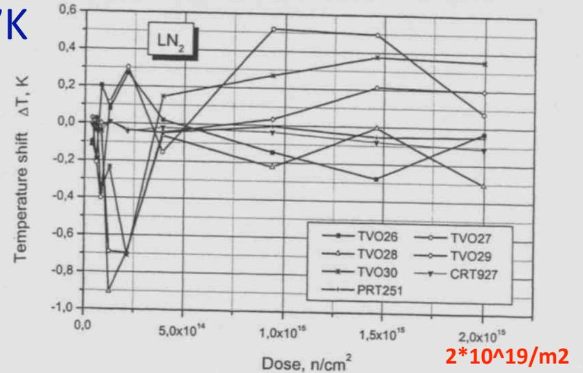
FIGURE 1. Temperature shift due to neutron irradiation in LN<sub>2</sub> at flux of about  $10^{10}$  n/(cm<sup>2</sup>s) versus the total dose for TVO and CRT-2 sensors ( $D_\gamma = 85$  kGy).
