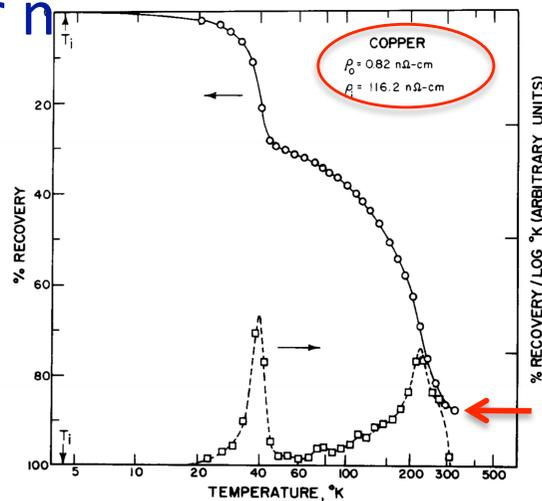
Fig. 5. Recovery and differential recovery versus logarithm of absolute temperature for copper irradiated at 4.5 K to  $2 \times 10^{18}$  n/cm<sup>2</sup> of  $E > 0.1$  MeV.
