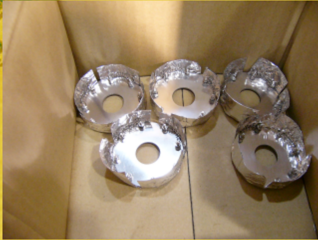
Al baffles with a center hole of 1/3 of cryo-pipe diameter
