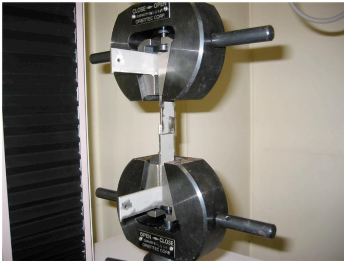
Tensile Lap-Shear Strength of GUG: Irradiated to 10 MGy in LN2
