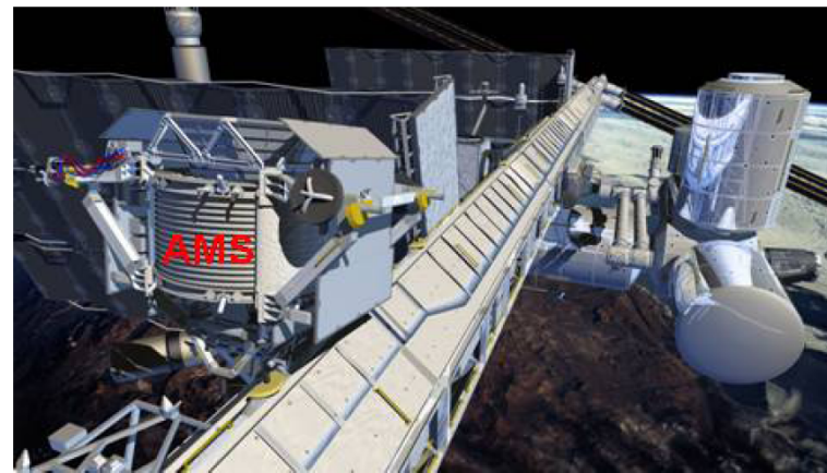
AMS-02 (Alpha Magnetic Spectrometer on ISS) Saturated He II in space (microgravity) 1.8 K
